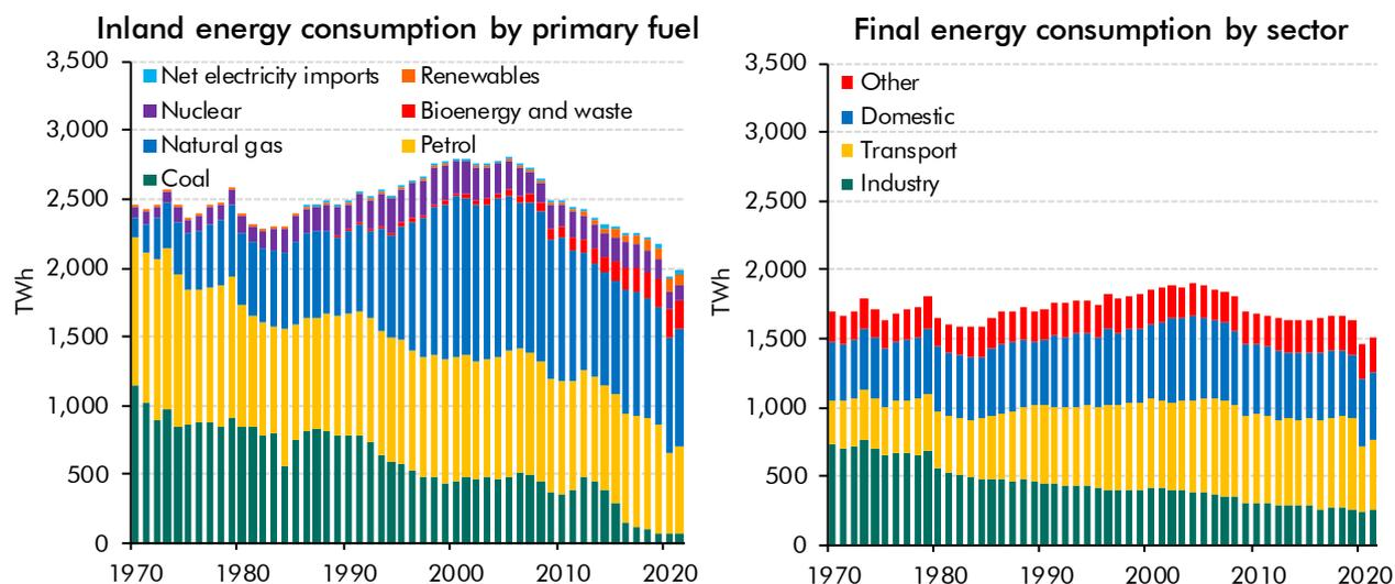
Note: The left hand chart is the UK's primary energy consumption by energy source. On the right is the final energy consumption by sector. The disparity is due to inefficiencies within the power system.
